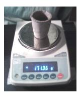
3) Transfer approx. 100g of oven dried material to the crucible and record mass of crucible + material to nearest 0.01g under "initial mass of crucible & sample."
