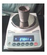
9) The percentage of organic carbon can be found by dividing the weight of the organic carbon found in the previous step by the dry weight of the material before burn off. Note that this is calculated differently than moisture content.
