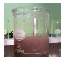
15) After each reading, gently remove the hydrometer and clean by placing it into the cylinder of distilled water and twirling it gently or by spraying it off with distilled water and wiping dry with a paper towel. Then, gently insert a thermometer into the suspension and record the temperature.
