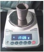
Transfer approximately 100g of material from the container to the crucible, weigh the filled crucible, and record this weight under "Weight of Crucibles and Unburned Sand (g)."
