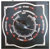
15. When the furnace has heated to between 800°F and 850°F, turn the temperature setting to between 4.6 and 4.8, and press the **start** button again.
