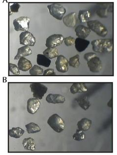
**FIGURE 1:** Sand with high percentage of quartz (~80%). A) Before abrasion resistance test and B) after.
