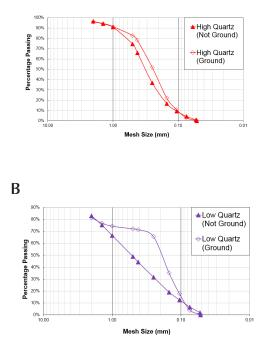
**FIGURE 3:** The amount of change in a track material as a result of abrasion resistance testing. A) Sediment with a high percentage of quartz (approximately 80%), and B) low percentage of quartz (approximately 3%).
