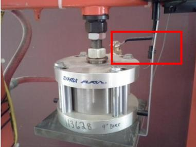
11) Move the assembly to the orange **test frame** and connect the upper transducer wire to the **Pulsar box** in the "T/R" transmit receiver port.
