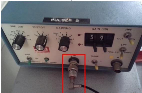
Connect the **lower transducer** wire to the left port in the
