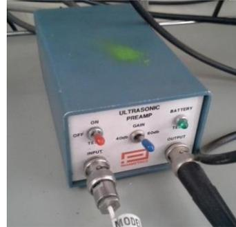
Be sure the wire from the "out" port on the preamp is connected to the left-side "Channel 1" (CH1) port of the **oscilloscope**. Also, be sure the wire from the back side of the pulser is connected to the right-side trigger port of the oscilloscope (EXT TRIG).
