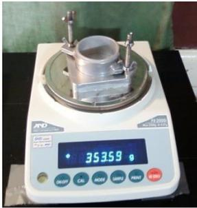
7) Attach the **top half of the proctor**. Fill the proctor with sample, taking care not to compact it.
