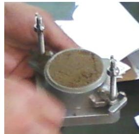
11) Weigh the bottom part of the proctor and the sample to  $\pm 0.01\text{g}$ . Record this weight on the data sheet under "Weight of the mold and the wet material."
