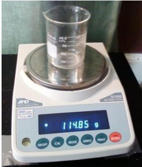
13) Place the entire sample from the bottom half of the proctor into the sample tin (or beaker). Weigh the wet sample to  $\pm 0.01g$ , record the weight under "weight of container + wet material", and place the tin into the oven (or microwave oven). Work quickly because water is being lost as time progresses.
